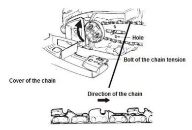
6) Adjust the chain tensioning nut in the lower hole of the guide. Then install the chain and secure the mounting nut.
