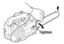
While lifting the chain guide, turn the content screw to apply correct tension to the chain.
