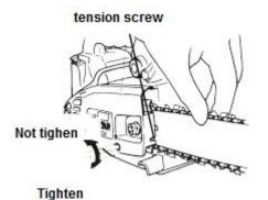
8) Tighten the nuts and check if the chain is rotated correctly and tight.
